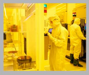
The C2MI MEMS laboratory has class 10 and class 1 clean rooms on the surface of the slices. The infrastructure is suitable for the micro-machining of surface layer as well as silicon. The C2MI features production lines for first-level assembly as well as MEMS fabrication and advanced packaging on 200mm slices.
