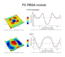
This technique usually requires sample preparation. BGA removal, bake and application of a thin layer of high-heat white paint are recommended in order to obtain optimal results.
