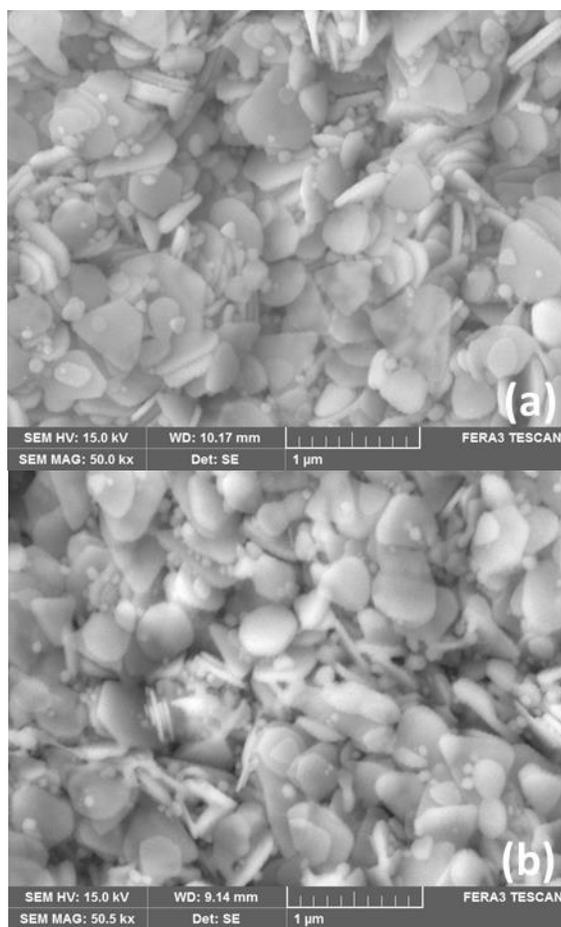
**Fig. 11** : SEM picture of silver ink particles before (a) and after (b) HAST
