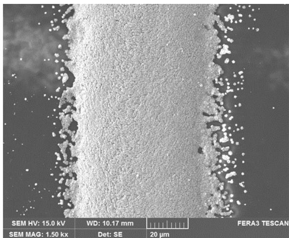
Fig. 2 : Chemical contrast view of the silver ink lines overspray
