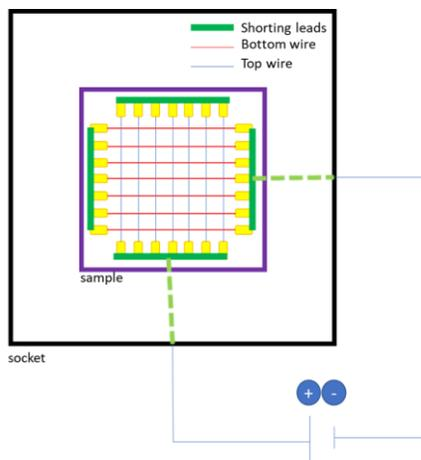
Fig. 5 : HAST electrical setup
