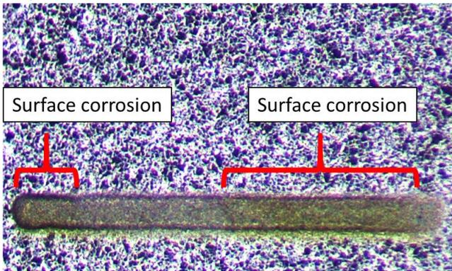
Fig. 7 : Surface corrosion on silver ink
