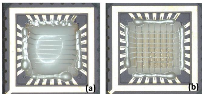
Fig. 3 : Printed wire bonds array with (a) epoxy and (b) polyimide
