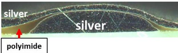
Fig. 8 : Cross-section view of silver inks lines crossing over
