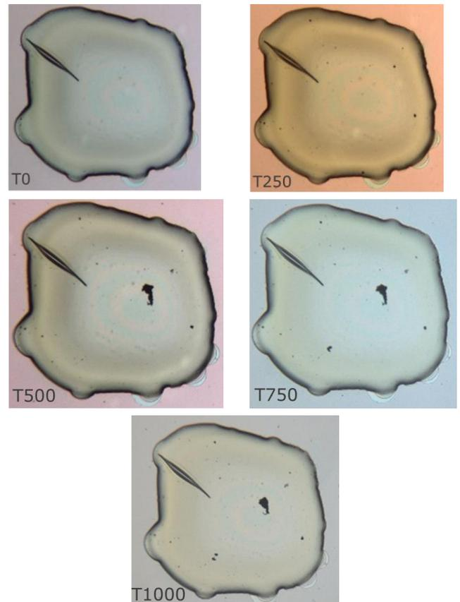
Fig. 6 : Cracking remains unchanged throughout DTC on polyimide ink dot
