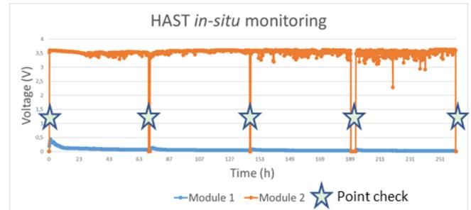
Fig. 9 : *In-situ* HAST monitoring
